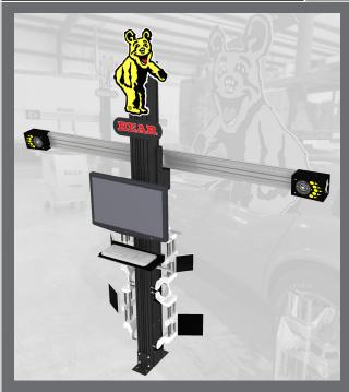
The Dimension 4 can also be configured without a roll—around cabinet. This model has all computer peripherals self contained to use minimum shop space without sacrificing functionality. Rim clamps and target are neatly stored on the system's main column.
