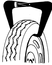
Figure 5.6 – Measuring wheel width with a caliper
