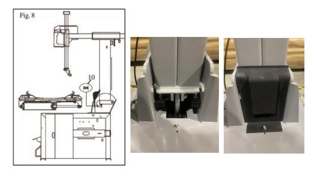
• Set the blade (R) on the bead breaker arm. Place the washer (15) inside the arm and the washer (16) outside. Fig. 9. Tighten the self-locking nut (17) on the blade pin. Fig. 9/A
