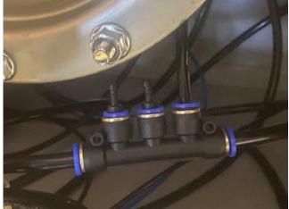
Re-mount the filter assembly in the back of the assist arm and re-connect the pneumatic hoses that were labeled in a previous step, as shown below.
