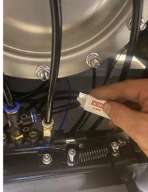
Connect the pneumatic valve that came from the assist arm in-between the two hoses that were spliced, as shown below.
