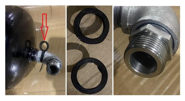
• Tighten the union and fasten the screws to attach the tank's bracket onto the machine.
