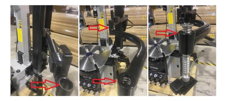
Mount the lower assist arm that has the rotating disc, as shown below. (Lubricate the areas that connect with white grease).
