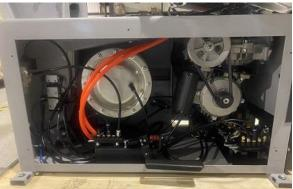
• Pull out the main power cable from the inside of the machine though the larger hole in the back. Be careful and avoid entanglement of this cable in the interior of the machine, which could result in disconnection of an airline.
