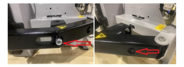
• Swing and remove the bead breaker arm, insert the rubber cushion.
