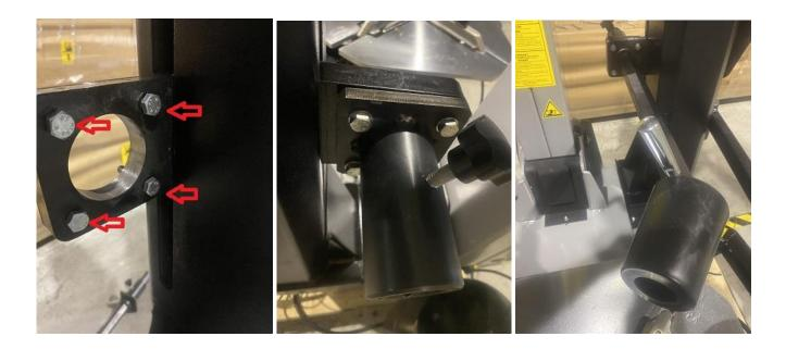
Pull out the pneumatic hose and valve that are rolled inside the assist arm's body. Disconnect the valve and route the hose through the hole in the side of the machine. Reconnect the valve inside the machine, as shown below.
