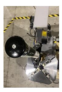
• Remove top locking nut from the spring base and tighten flat nut existing lower locking nut. Insert / mount plastic protector and fasten locking nut.
