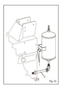
• There is a supply of two (2) O-rings (gaskets) attached to the air tank. Use one to attach the hose onto the tank's union and save the other one for future use if required.
