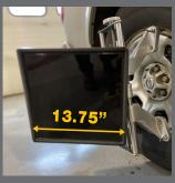
The Dimension 4 imaging cameras gain readings from the high resolution targets mounted on each wheel. Inside the targets are high precision 'mirrors' that are manufactured using a state-of-the-art printing technology that offers unbeatable resolution for extremely high accuracy. Each target is mounted on a light weight, durable aluminum, self-centering clamp adapter with a range from 12" up to 24" wheels.
