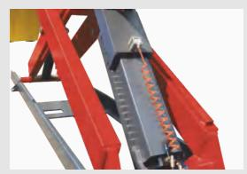
Mechanical lock and air-driven safety release.
